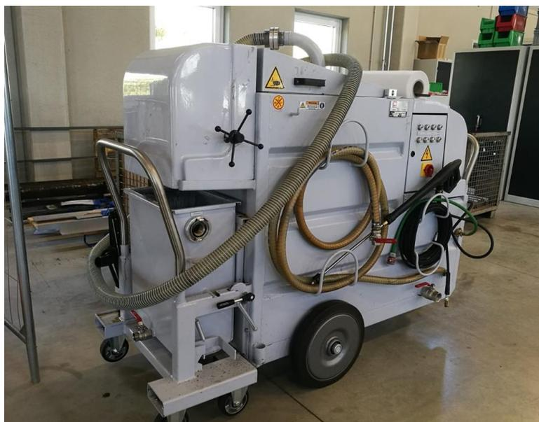
Illustration of Vacuum filter device
